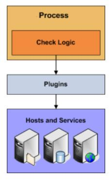
Active checks are initiated by the check logic in the Shinken daemon. When Shinken needs to check the status of a host or service it will execute a plugin and pass it information about what needs to be checked. The plugin will then check the operational state of the host or service and report the results back to the Shinken daemon. Shinken will process the results of the host or service check and take appropriate action as necessary (e.g. send notifications, run event handlers, etc).
